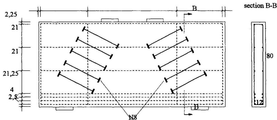
Fig. 2 – Beam 7/S strengthening reinforcement detail
