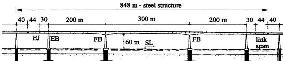
Legend: EB = Expansion Bearing; FB = Fixed Bearing; EJ = Expansion Joint; SL = sea level
