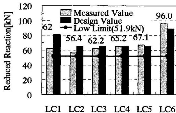
Fig.3 : Reduced Reaction in Gerber Hinge Support
