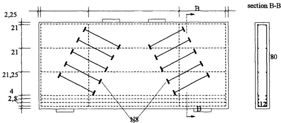
Fig. 2 – Beam 7/S strengthening reinforcement detail
