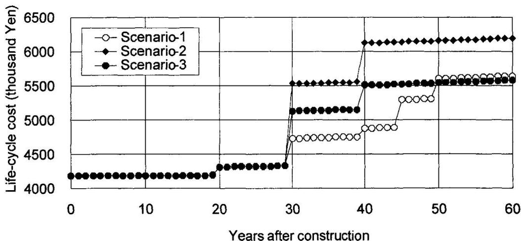
Fig. 3 Life-cycle cost calculation with three scenarios
