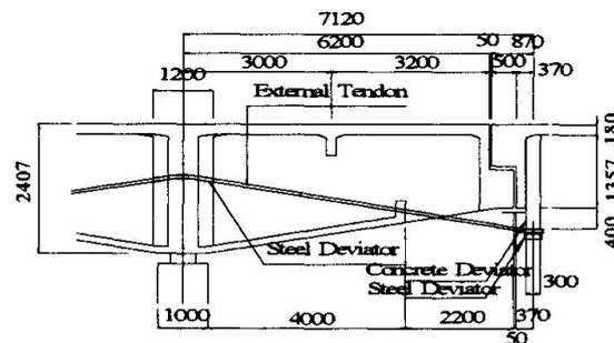
Fig.2 : Cable Arrangement at Gerber Hinge
