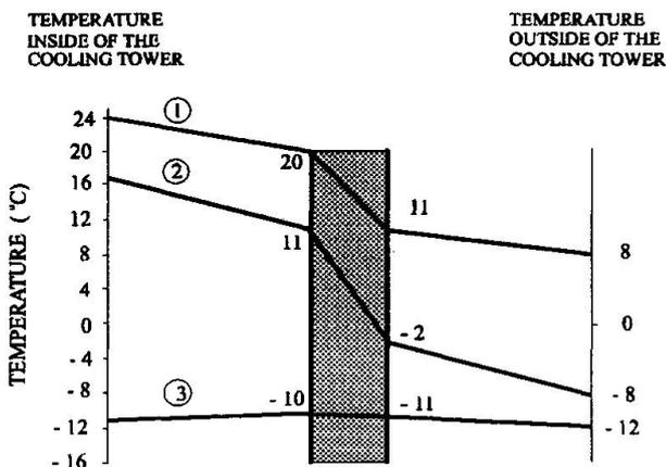
Fig. 1 Temperature profiles through reinforced concrete shell
