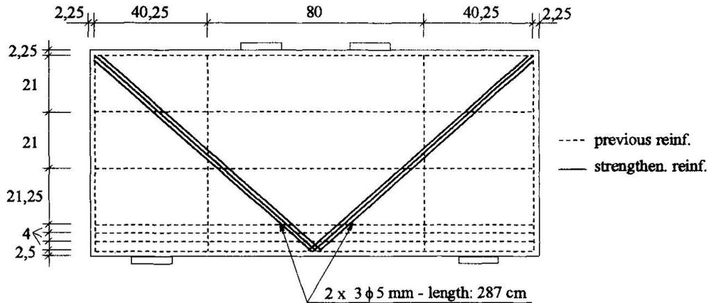
Fig. 1 – Beam 5/S strengthening reinforcement detail (cm)
