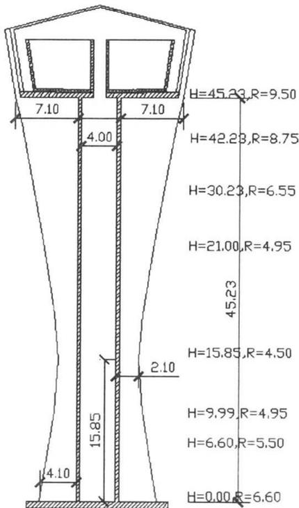
Figure 1 Water tower-Model 1
