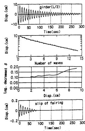
Fig.-1 Free vibration and damping
