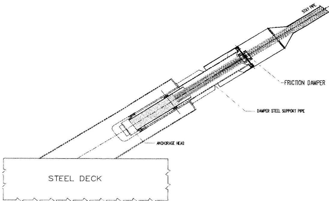
Figure 1. Installation of friction damper on UDDEVALLA Bridge
