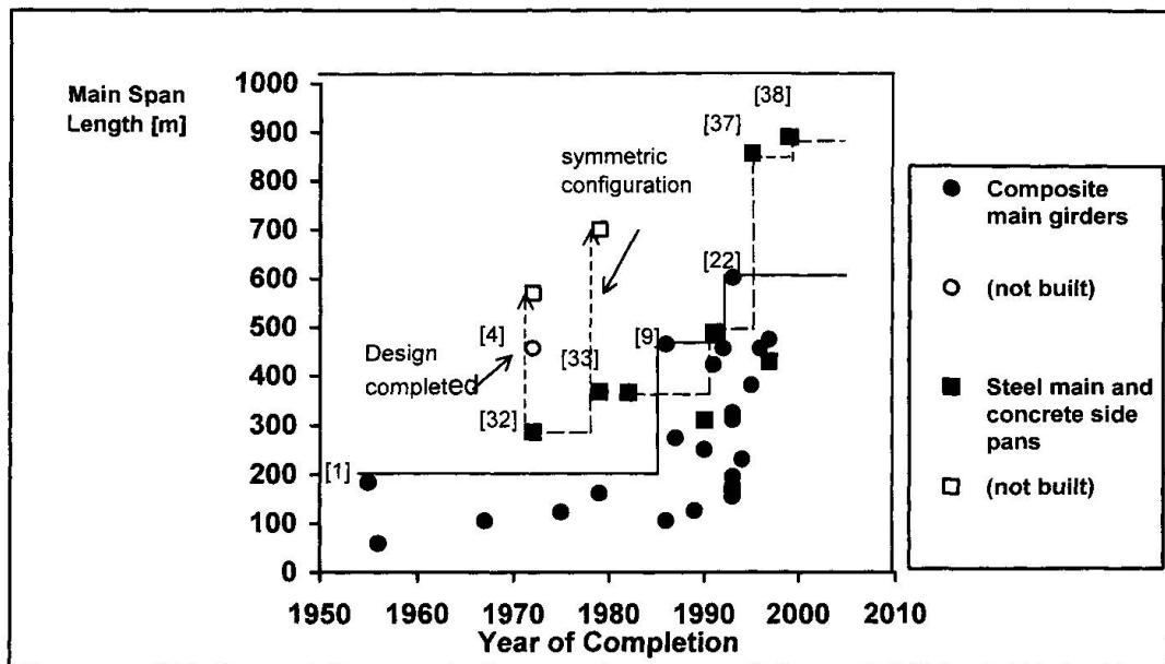
Figure 1. Development of span lengths, from Tables 1 and 2
