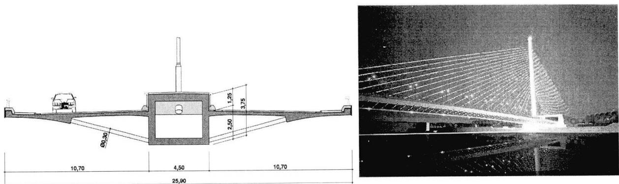
The main span of the bridge over the river is 162 m long, in continuity with a short 31 m long span above the left embankment and a very short 12 m long span between the pylon and the balancing abutment. This abutment is 122 m long and is the first part of a tunnel that goes on under the railway junction.
