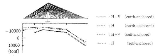
Fig. 4 Axial force of main girder
