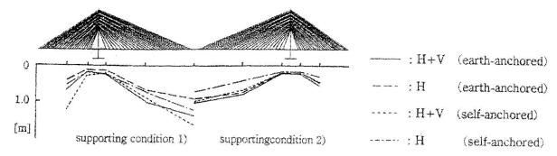
Fig. 3 Maximum vertical displacement of main girder
