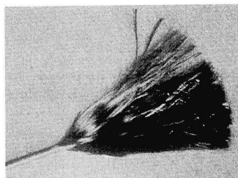
*Fig 3. CFRP wire, 5mm diameter, with
