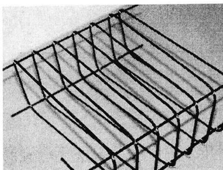
*Fig 2. CFRP bars and stirrups,
