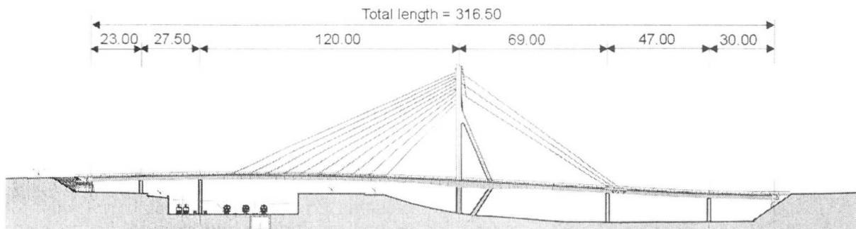
Fig. 3 – A cable-stayed viaduct in Oporto.
