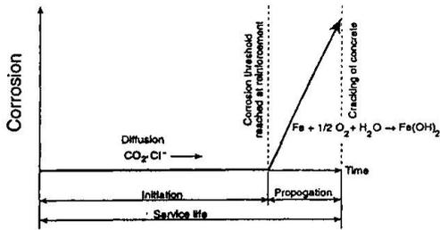
Figure 3 Corrosion model proposed by Tutti <sup>(9)</sup>
