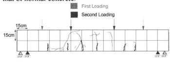
Fig. 5 Crack Pattern of Series B (Normal Concrete, Water Curing)
