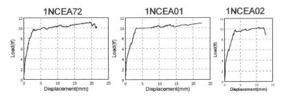
Fig.4 Load-Displacement Relationship at the center of the span (Expansive Concrete)
