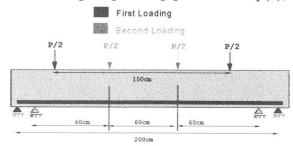
Fig. 2 Loading System for Series B
