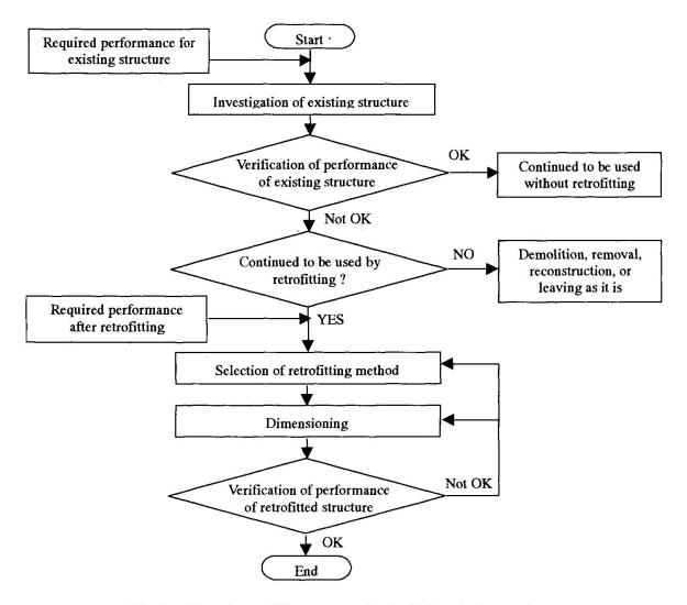
Fig.1 Flowchart of the proposed retrofitting design system
