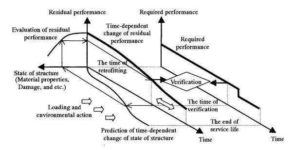
Fig.3 Verification of performance along the time
