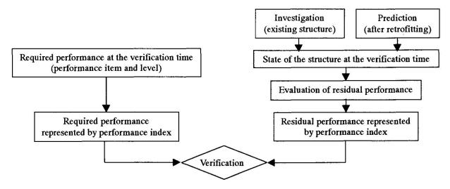
Fig.2 Verification of performance using performance index
