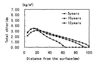
Fig.6 Chloride profile in cover
