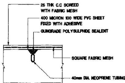
**Fig. 5 : Typical Joint between Precast units in Longitudinal Direction**
