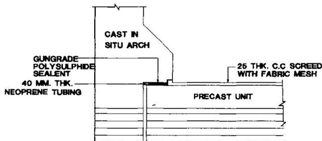
**Fig. 6 : Details of Joint between Precast Unit and Cast-in-Situ Arch**
