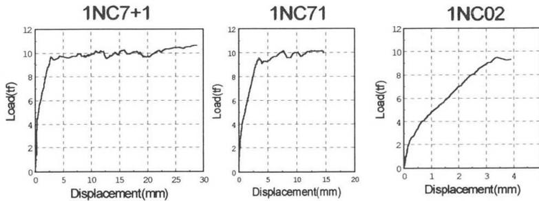
**Fig.3** Load-Displacement Relationship at the center of the span (Normal Concrete)
