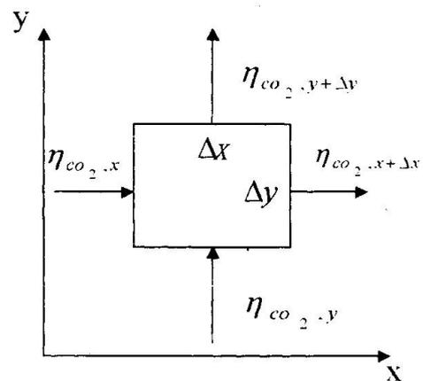
**Fig. 2 CO<sub>2</sub> mass flux in the x- and y-direction**
