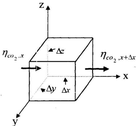
**Fig. 1 Mass flux of x direction in a three-dimensional control element**
