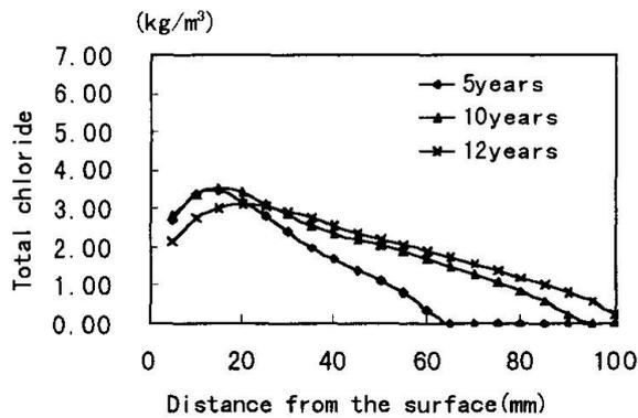
Fig.6 Chloride profile in cover
