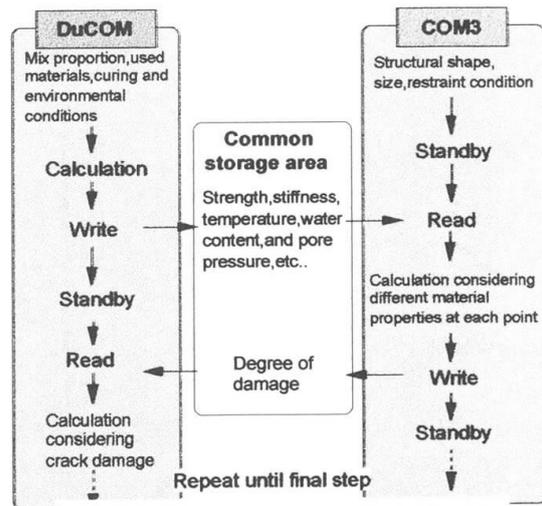
Fig.6 Parallel Processing of DuCOM and COM3
