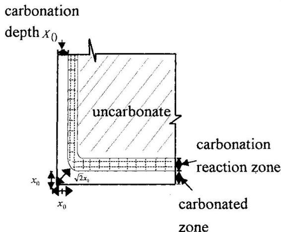
Fig. 3 Carbonation distinguish of concrete
