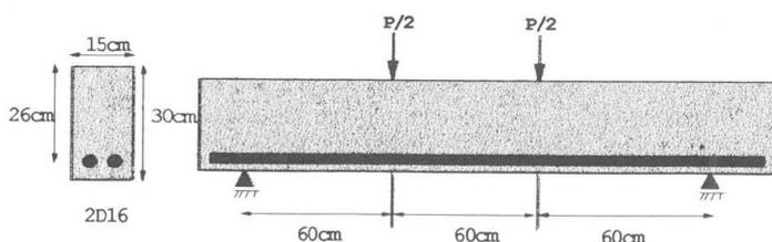
*Fig.1 Geometry of the beams and Loading System*
