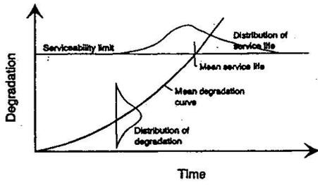
Figure 1 Degradation of concrete structures <sup>(8)</sup>
