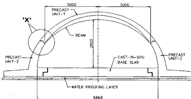
Fig. 1 : Precast Subway showing different Units
