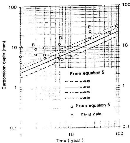
Figure 4 Comparison of carbonation depth with field data
