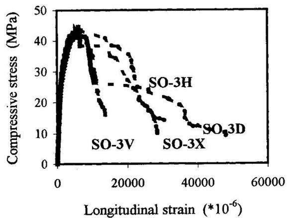
Fig. 1 Compressive stress-strain curves for circular columns
