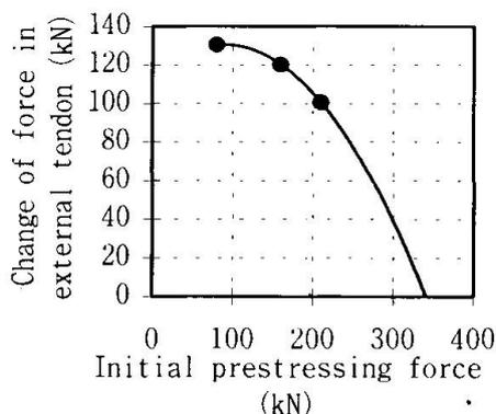
Fig.4 Relationship between Change in Tendon Force and Initial Prestress
