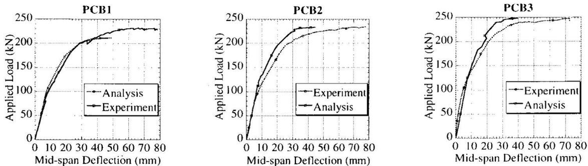
Fig.5 Comparison between Experimental and Analytical Load-Displacement Relationships
