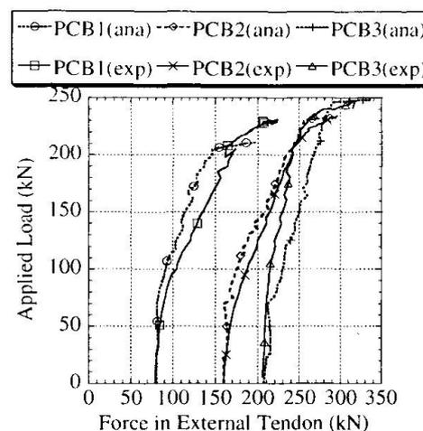
Fig.3 Analytical and Experimental Characteristic of Tendon Force
