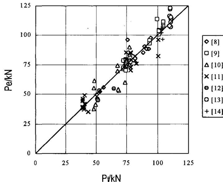
Fig.2 Comparison of calculated and experimental shear resistance
