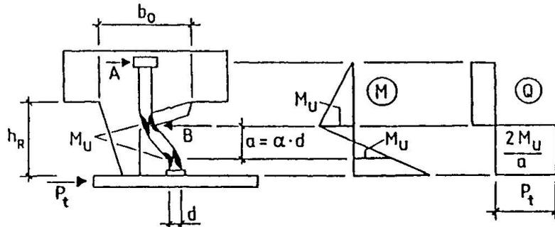
Fig.1 Failure Mechanism of stud used with profiled steel sheeting
