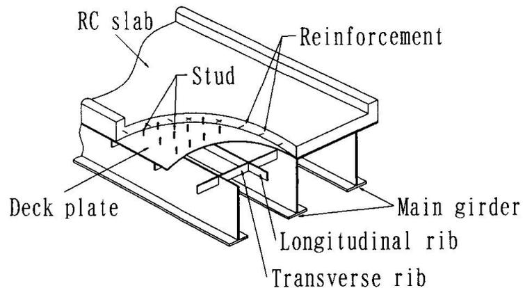
Fig.1 General view of modified composite deck girder
