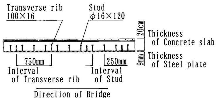
Fig.3 Section of real-size model
