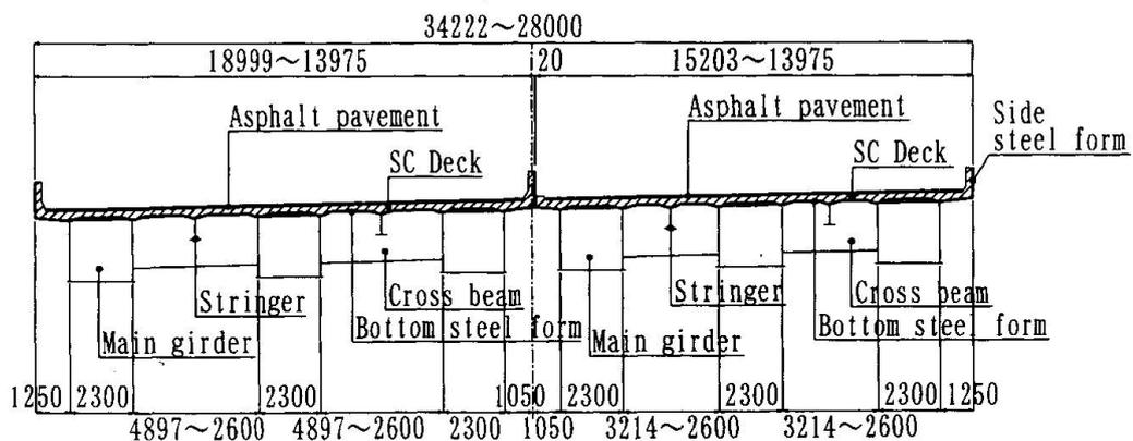
Fig.5 Typical cross section of the Kariyasuga Viaduct
