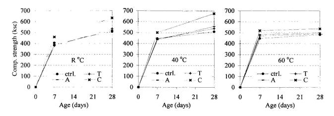
Fig. 4 Type of fly ash on compressive strength at 20% replacement (W/B = 0.45)
