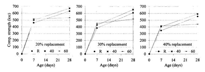
Fig. 3 Effect of temperatures on compressive strength for fly ash C concrete (W/B = 0.45)
