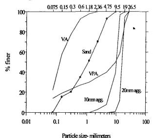
Figure 2: Particle size distribution
