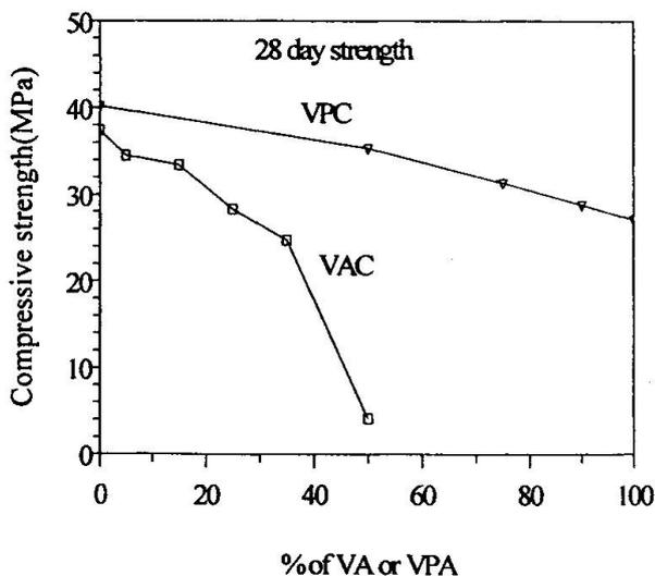
Figure 3: Compressive strength of VAC or VPC
