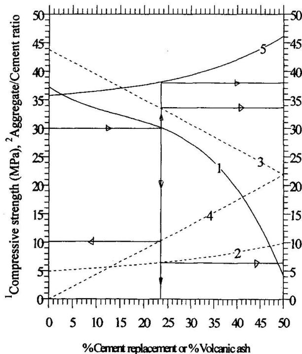
Figure 5: Typical mix design chart for VAC
