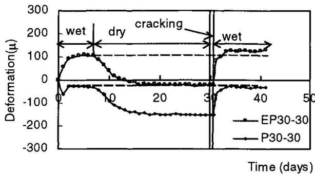
Fig.5 Deformation of specimens under drying and wetting
