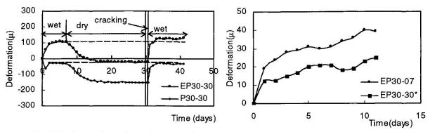
Fig.5 Deformation of specimens under drying and wetting
