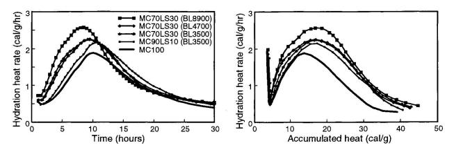
Fig. 1 Accelerated hydration heat of cement in terms of time and accumulated heat [5]
