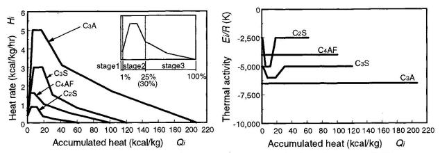
Fig.2 Reference heat rate and thermal activity of each mineral compound [7]
