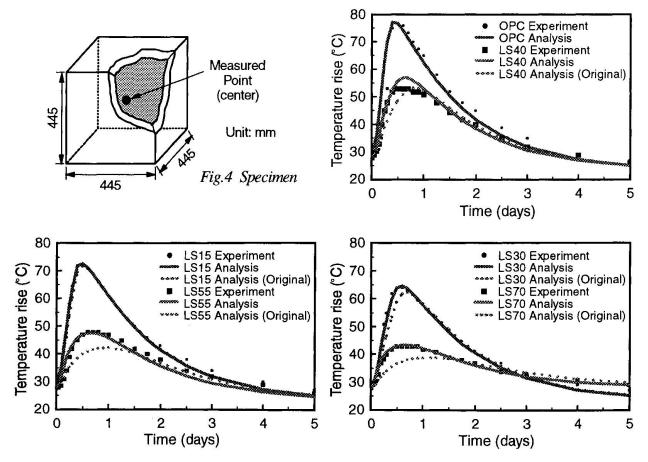
Fig.5 Comparison between analysis and experiment
