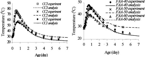
Fig. 5 Temperature in plain concrete specimens Fig. 6 Temperature in concrete with fly ash FAA
