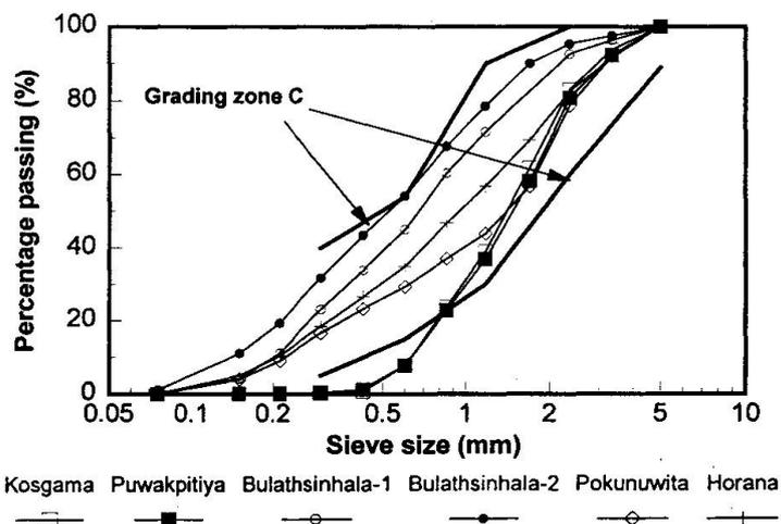
Fig.3 Particle size distribution of Land based sand
