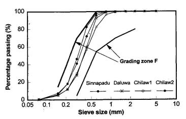
Fig.2 Particle size distribution of Dune sand
