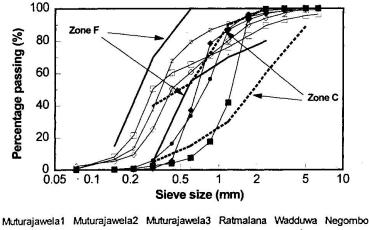
Fig.1 Particle size distribution of offshore sand
