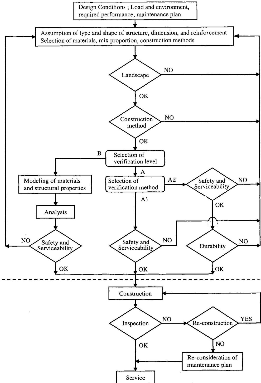
Fig. 1 Framework of integrated design(3)
