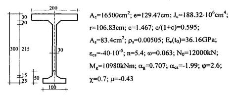
Fig. 4 Prestressed post-tensioned section
