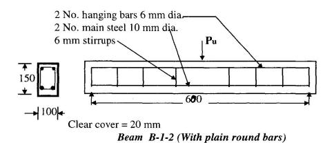
Fig. 1 Typical Details of Test Beams for Static Loading
