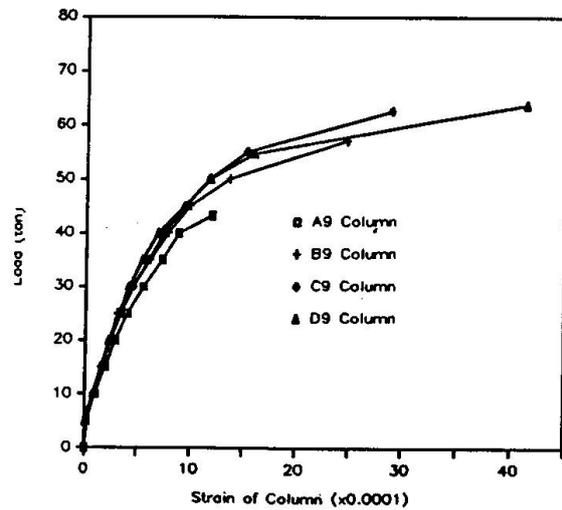
Fig. 7 Relationship between load and strain of columns under eccentricity of 9 cm
