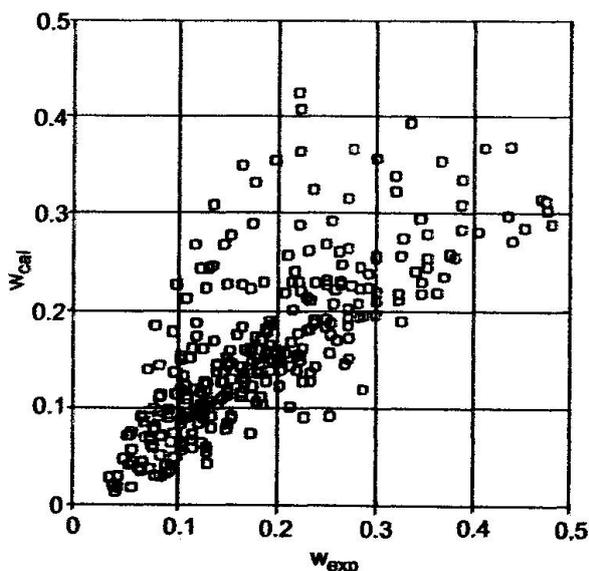
Figure 4 Crack width - calculated versus measured values [5]
