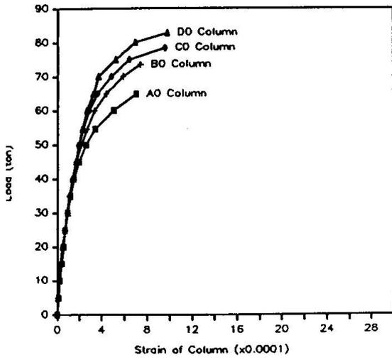
Fig. 4 Relationship between load and strain of columns under concentric loading
