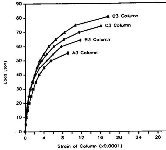
Fig. 5 Relationship between load and strain of columns under eccentricity of 3 cm
