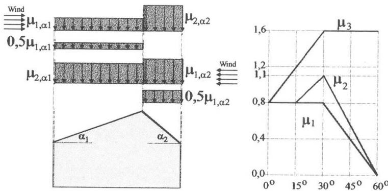
This may be illustrated by the following example: snow loads. In the past, only a constant load had to be considered in the design of buildings in Germany. The new EC 1 part 7 [4] requires 4 different load cases. This arrangement of loads is more realistic than a constant load. But does it lead to an increase in safety?
