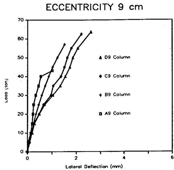
Fig.11 Relationship between load and deflection of columns under eccentricity of 9 cm
