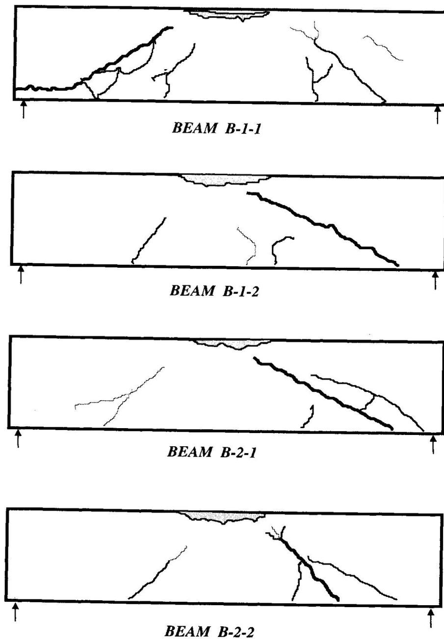
*Fig. 2 Cracks and Failure Pattern of Beams Under Flexure*
