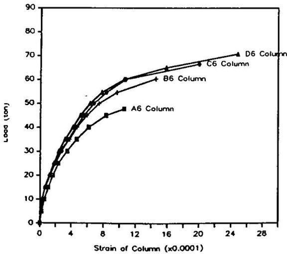
Fig. 6 Relationship between load and strain of columns under eccentricity of 6 cm
