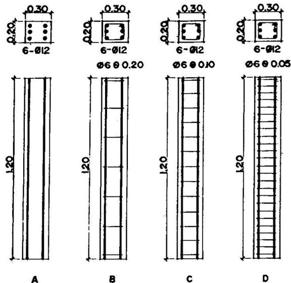
Fig. 1 Detail of main and tie bars of reinforced concrete columns
