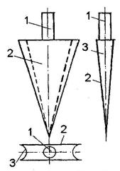
Fig. 2 Tip for penetration of soils with anisotropic properties: 1- tang; 2- working facets; 3- side facets
