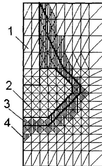
Fig.4 This is an example of the calculated sphere of cast-in-situ piles in punched hole during of numerical modeling its work: 1- shaft; 2- hard widening; 3- compaction zone; 4- zones of plastic deformations
