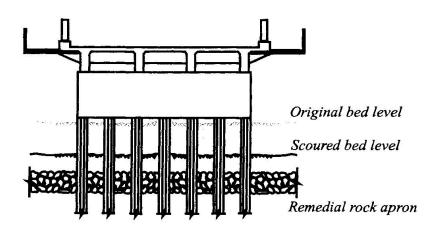
Figure 1 Typical Side Elevation of a Foundation and Remedial Works for the Ashburton River Road Bridge
