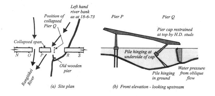
Figure 3 The Bulls Road Bridge Failure
