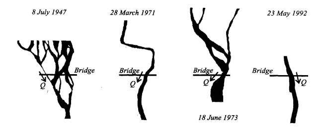
Figure 2 Development of the Principal Flow Channels of the Rangitikei River at the Bulls Road Bridge
