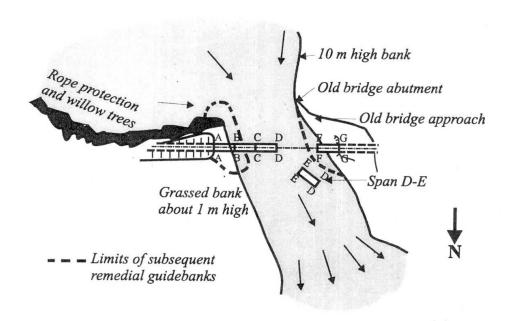
Figure 4 Schematic Site Plan of the Waitangitaona River Road Bridge Failure
