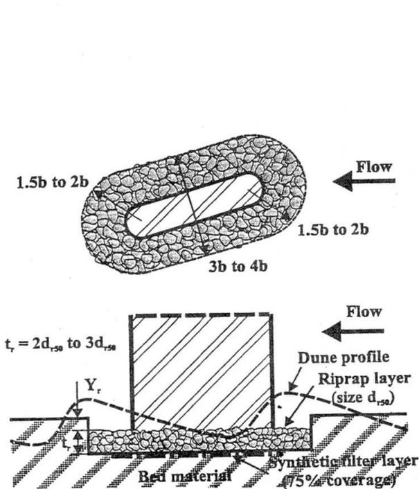
Figure 3 Riprap Placement Recommendations
