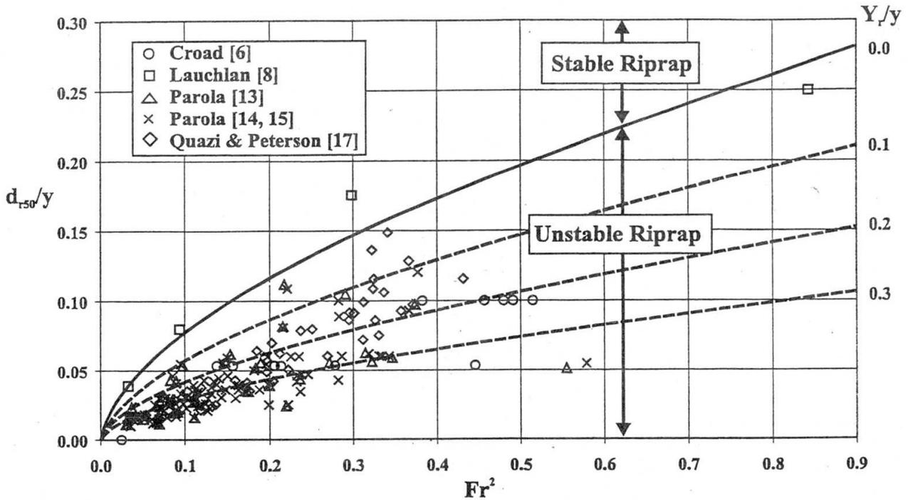
Figure 2 Design Curves for Riprap Size by Lauchlan [8]
