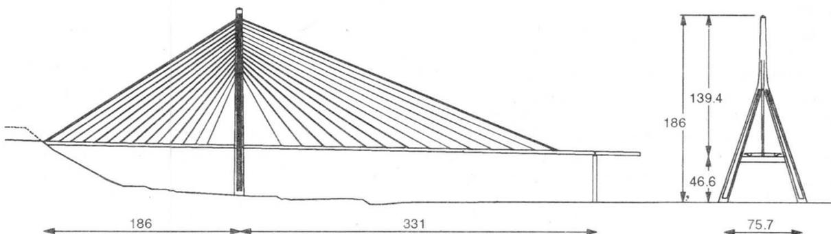
Fig.2 Bridge Elevation
