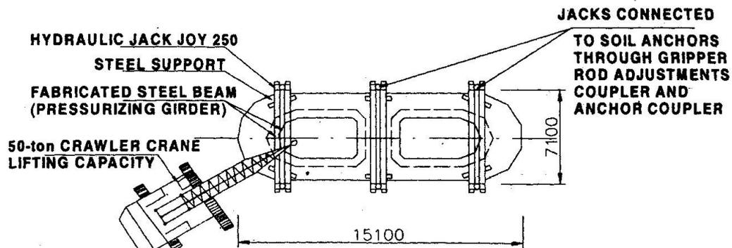
Fig. 3 : Arrangement of jack down method
