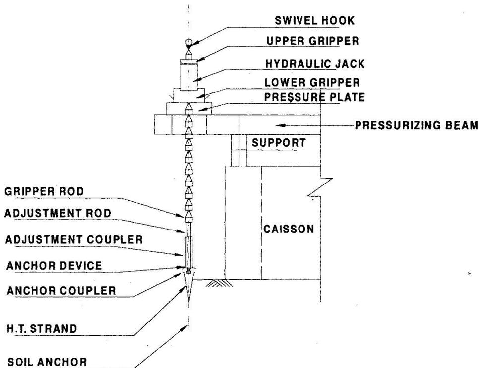
Fig.5. Components of jack down method
