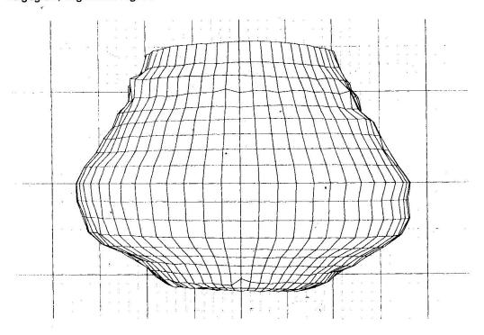
Fig. 5 Graph showing dimensions and shape of borehole enlargement
