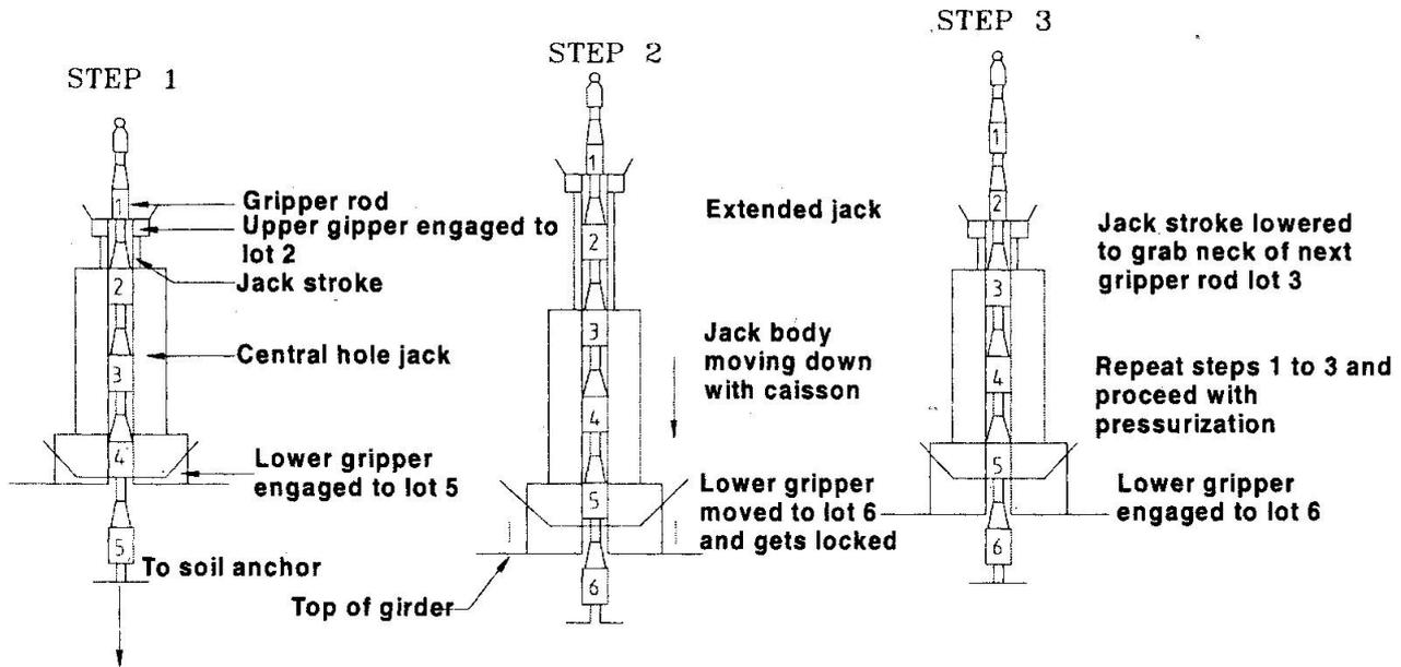
Fig. 4. Pressurizing mechanism to jack down the caisson
