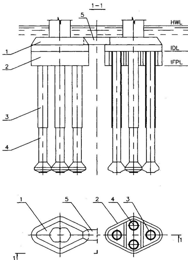
Fig. 1 General arrangement of foundation: 1 – pile cap, 2 – ice protective shell; 3 – steel encasement; 4 – bored pile; 5 – strut; HWL – high water level; IDL – ice drift level; IFPL – ice first push level (min)
