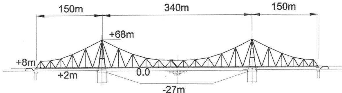
For the third time a swing bridge over the Suez Canal at El Ferdan (Egypt) is under construction. After completion it will be the largest moveable bridge in the whole world, and this bridge will reinstate the former road and rail link across the Suez Canal.
