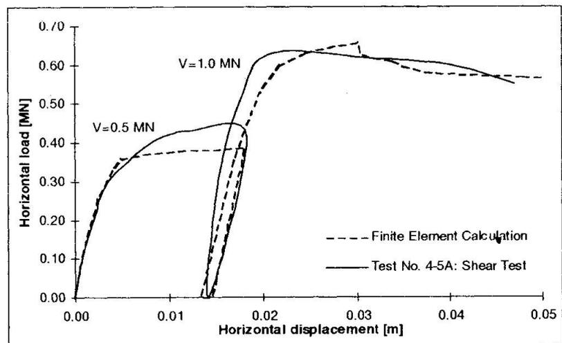
Fig. 4: Calibration to medium scale shear plate test, [3]
