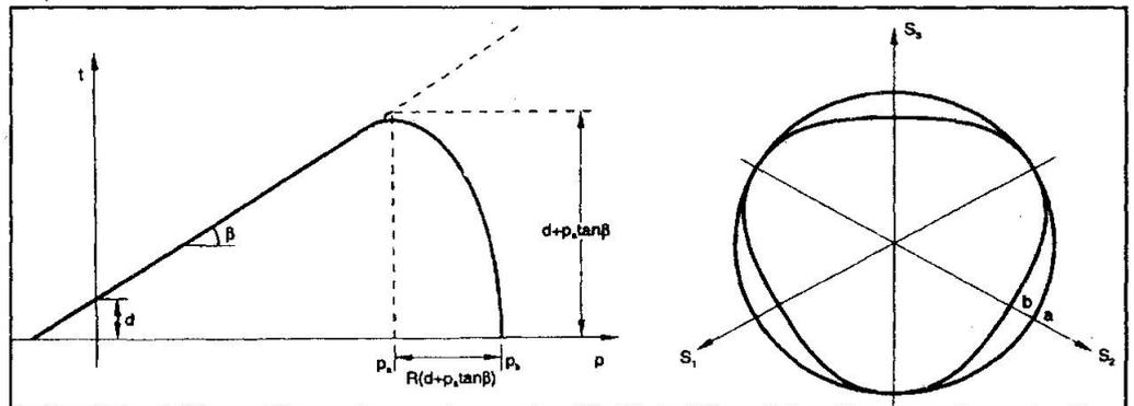
Fig. 3: Drucker-Prager model with cap as defined in ABAQUS, [2]
