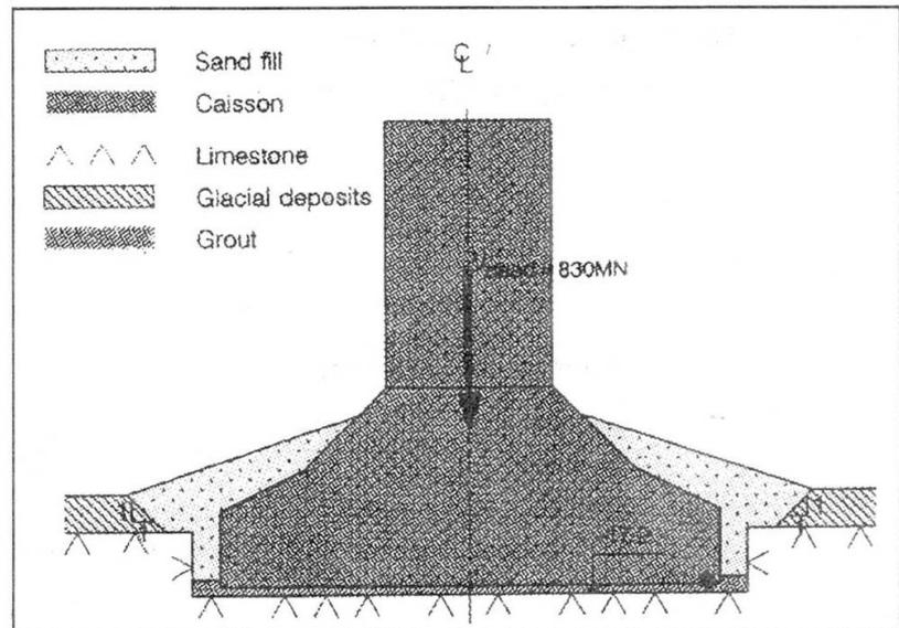
Fig. 1: Geometry and foundation conditions for pylons
