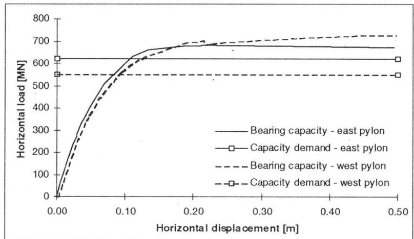
Fig. 5: Load-displacement curve for east and west pylon
