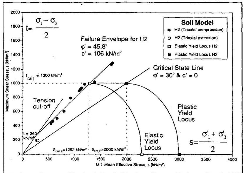
Fig. 2: Principle soil model for Copenhagen Limestone, after [3]
