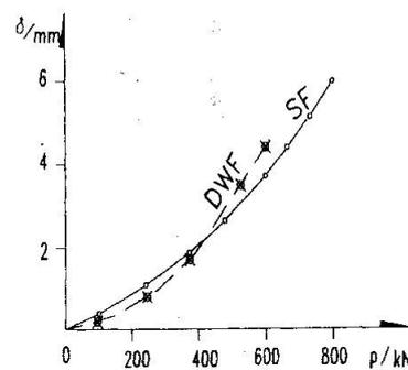
*fig.5 P- delta curve when horizontal loading*
