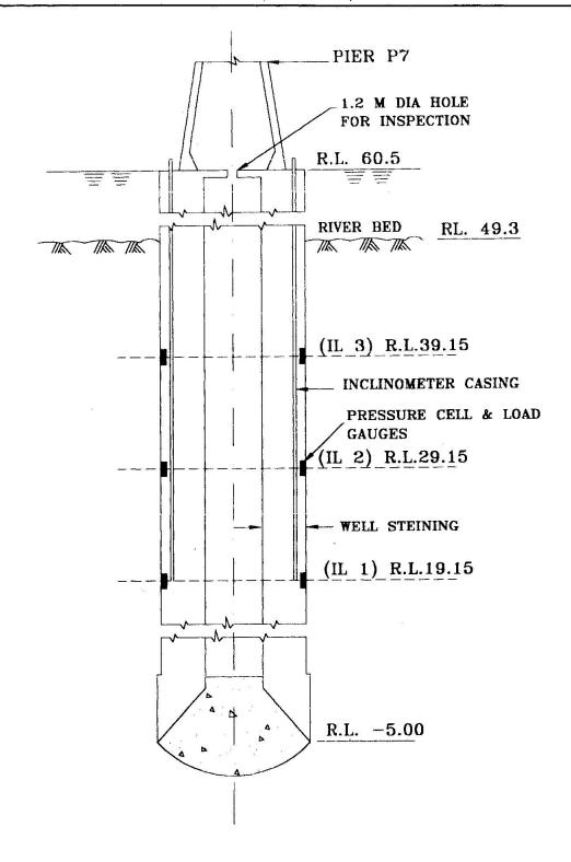
FIG.2 INSTRUMENTATION LEVELS (IL) OF WELL P7 (SCHEMATIC)
