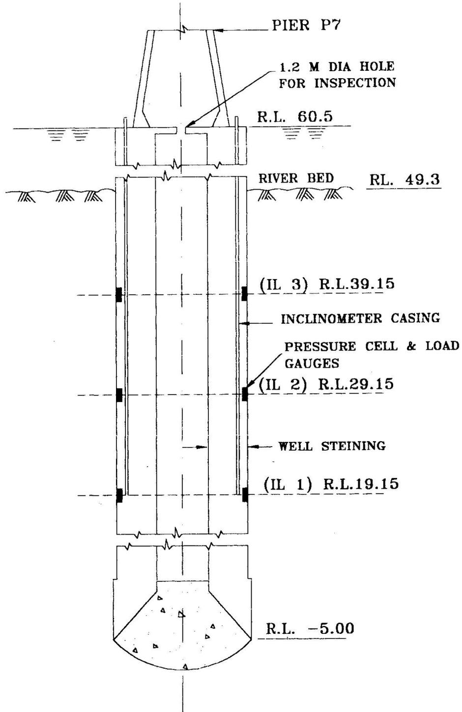
FIG.2 INSTRUMENTATION LEVELS (IL) OF WELL P7 (SCHEMATIC)
