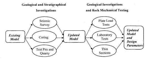
Fig. 2 Methodology for Establishment of Geology and Parameters
