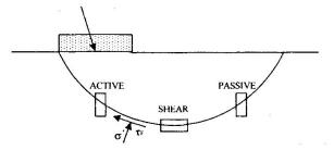
Fig. 6 Principal Failure Conditions
