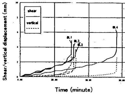
Fig.7 Relationship between time and shear/vertical displacement (average)
