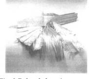
Fig. 1 Pultruded section showing glass reinforcement
