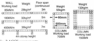
Walls, columns, beams, bridge girders, floors and roofs can be built using just three primary components pultruded from glass fibres and a suitable thermoset resin and insulating core materials. Structures can be designed using a fully developed limit state design method which is consistent with British and European building codes (1) (Fig 3).
