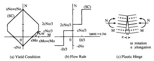
Fig.3 Yield condition and associated flow rule
