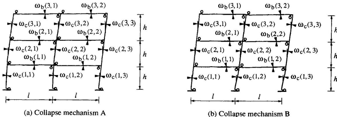
Fig.6 Collapse mechanism of 2-span 3-storied composite frame
