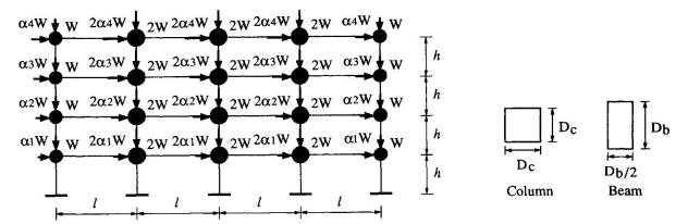
Fig.4 Composite frames subjected to vertical and horizontal loads
