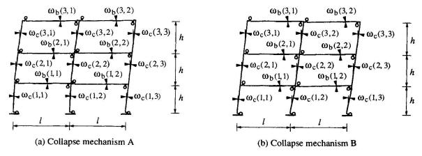
Fig.6 Collapse mechanism of 2-span 3-storied composite frame
