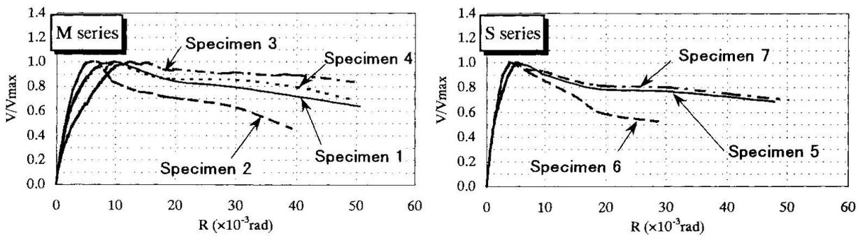
Fig.4 Envelopes of Horizontal Load-Story Drift Angle Curves
