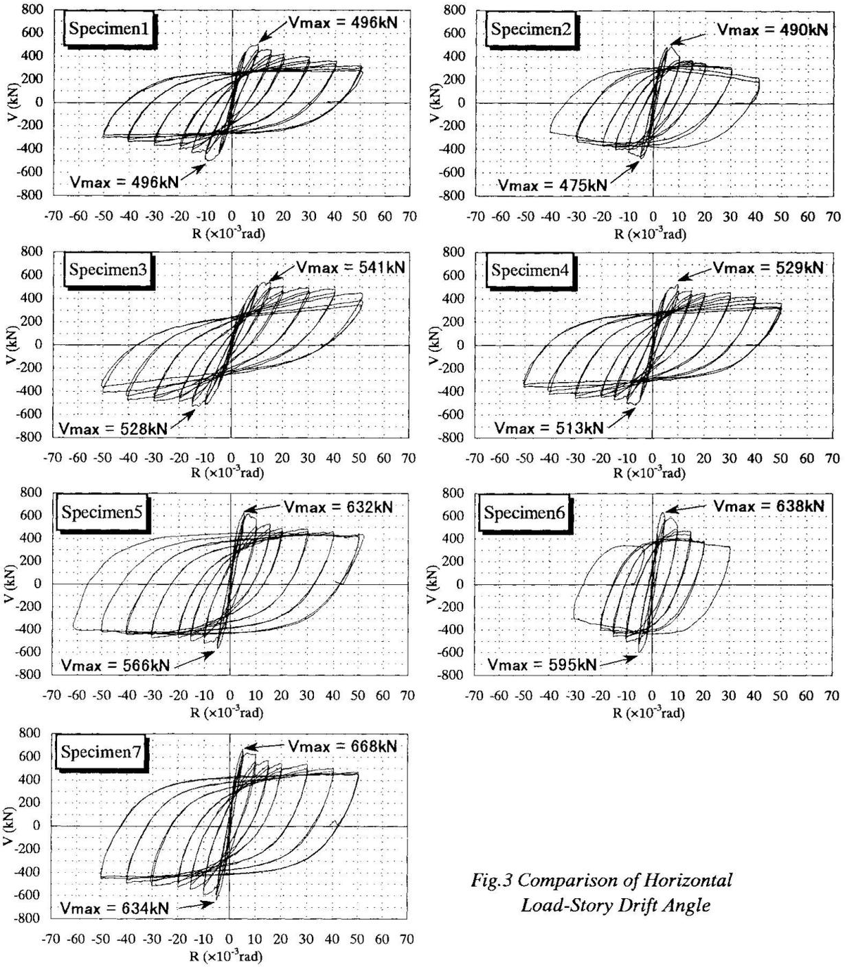
Fig.3 Comparison of Horizontal Load-Story Drift Angle
