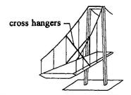
Fig.-3 Box girder with cross hangers
