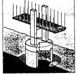
Fig.-4 Twin-shaft type foundation (left) and cylindrical solid foundation (right)
