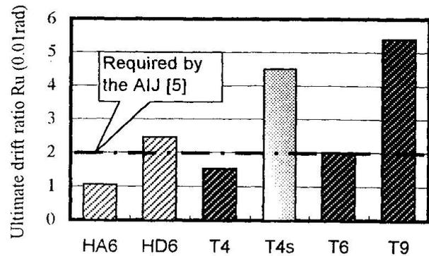
Fig. 3 Ultimate deformation
