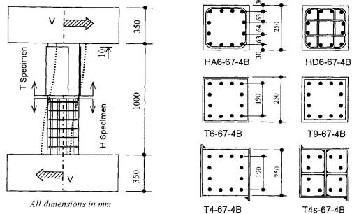
Fig. 1 Details of test specimens
