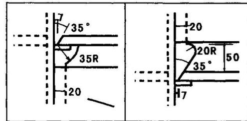
Fig.4 Weld Access Hole Details
