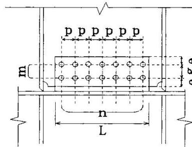
Fig.2 bolted web connection details
